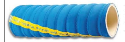
The Model RC2 Gamma top quality UHMW chemical suction/discharge hose with corrugations for superior flexibility and dual helix construction. For transfer of corrosive chemicals, acids, fuels and other chemicals.
